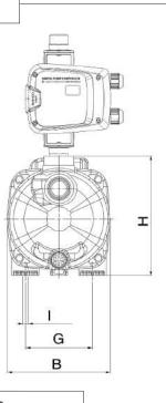
Height with controller fitted H2 + approx 228mm = 372mm
