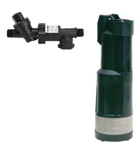
The RAINSAVERMK6 is an Automatic Rainwater / Mains Water Changeover Device designed to provide automatic mains back up for Pressure Pump supply systems. The RAINSAVERMK6 is designed to be installed in conjunction with a Pressure Pump supply system that is fitted with an independent pressure and flow controller with loss of prime protection and 24 hour auto restart.
