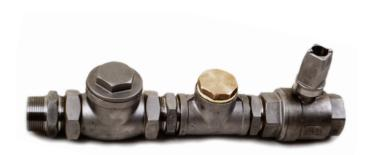
The boundary kit is generally located immediately adjacent to the front boundary of the property and allows the property to be isolated from the pressurised sewer pipeline in the street. The boundary kit comprises of a keyed isolation ball valve, swing check valve and an inspection tee arrangement.
